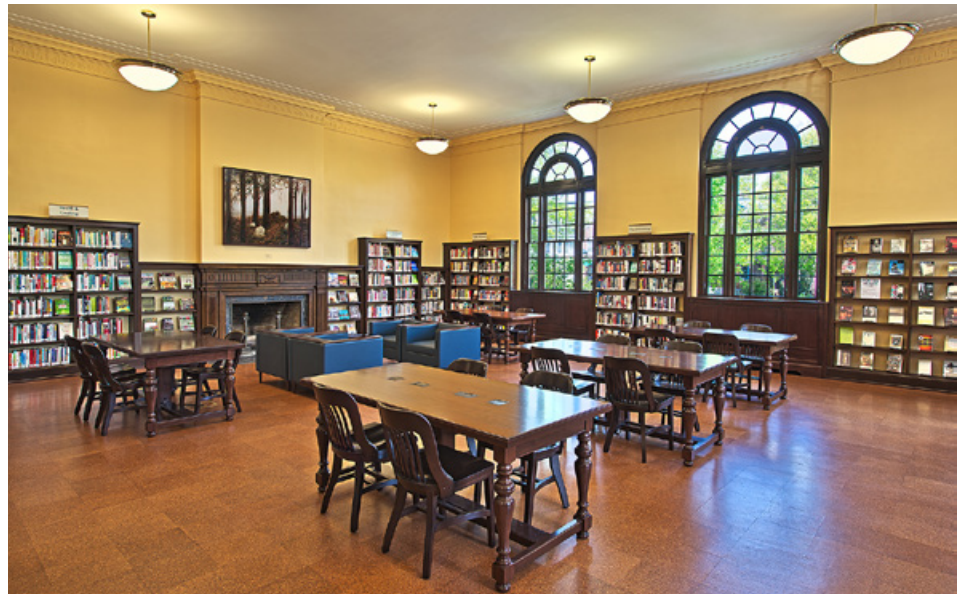
The terrazzo floor was restored, reading tables were adapted for computer use, the original woodwork restored, and lights that resembled the originals were installed.
